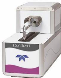
The LSS Boat Module is an ideal add-on to the Lotix TOC analyser. It uses high-temperature combustion to accurately measure carbon content in a variety of matrices, including soils, sludges, sediments, particulate-laden liquids and hard-to-oxidize samples. Analysis of 1 gram samples with up to 20mg carbon content can reduce errors associated with using small sample sizes. Switching between liquids and solids takes just minutes.
